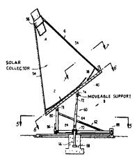
A solar concentrator is disclosed herein and includes a modularized point focusing solar concentrating panel which is movably mounted to track the sun. This panel has an overall parabolic reflecting surface and a triangular or approximately triangular configuration which improves structural integrity, minimizes wind resistance, and permits rapid and easy stowing.
