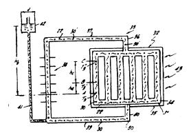
A solar heating system in which the heating transfer medium is circulated from the heat absorbing member through the heat exchange area by means of gravitational forces which are augmented by the use of a transfer medium containing additives which change in state from fluid to gaseous as they move through the system.
