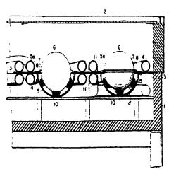
An apparatus for heating water by solar rays in which a plurality of spherical lenses are used to enable solar rays to be converged whenever there is sunlight present. Also incorporating a superheat resisting carbon impregnated cloth to cover that area of metal which is subjected to the intensive heat of the focused rays.
