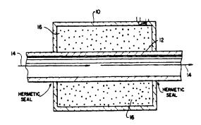
The disclosure relates to a solar radiation converting method and means whereby the addition of a halogen within a hermetically sealed space receives and converts solar or synthetic radiant spectra into heat energy; its principal advantage being the conversion of the visible portion of the light spectra into additional heat.
