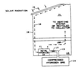
Thermal energy storage systems employing metal hydrides are useful for storing thermal energy produced, for example, by solar radiation. The metal hydrides, examples of which include FeTiH and the VH-VH<sub>2</sub> reaction system, evidence ease of reversibility of the metal
