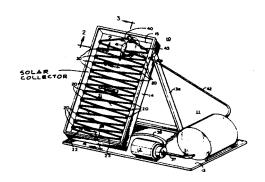
A solar heating system is provided which utilizes the sun's rays to heat fluid in a solar panel, which heated fluid is released to a storage tank when it reaches a predetermined temperature, and where it is available for withdrawal from the tank for heat exchange as desired.
