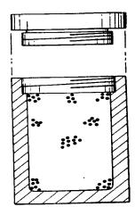
A thermal energy storage system comprising a germanium phase change material and a graphite container.
