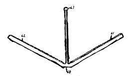
A solar concentrator with wide effective aperture is disclosed, which comprises at least one linear echelon reflector element which is inclined with respect to the direction of incident solar radiation to direct incident solar radiation to a line focus.
