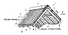
The invention relates to a roof and wall covering, in particular for heat-insulating house walls or roofs, consisting of board-like hollow plastic sections with several through profile chambers extending in longitudinal direction and of edge profiles insertable flush into each other.
