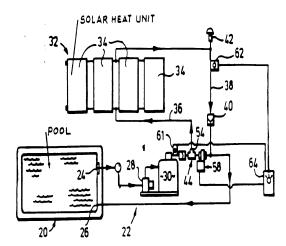
A solar heating system for a swimming pool and the like is disclosed. The system includes a circulation circuit having a pump by which water is withdrawn from the pool, passed through a filter, and returned to the pool. A solar collector assembly is provided and has flow and return lines connected in said circuit.
