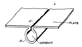
A solar collector which includes a radiation-absorbing panel having a surface provided with integral fluid-conducting conduits whereby heat absorbed by the panel may be efficiently transferred directly to fluid circulating in the conduits.
