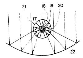
A device called Solar Trap for concentrating and collecting the solar energy is disclosed. Said Solar Trap employs, firstly, the principle of the light funneling as means for concentrating the sunlight and secondly, the principle of the repeated incidence as means for enhancing the absorption of the concentrated sunlight.
