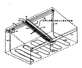
Solar heating system, wherein solar heating assemblies are adapted to form the roof of a structure. The solar heating assemblies may not occupy the entire surface area of a roof, but the upper sheathing elements of the solar heating assemblies may extend over the entire roof area so that no other provision for roofing of the structure is necessary.
