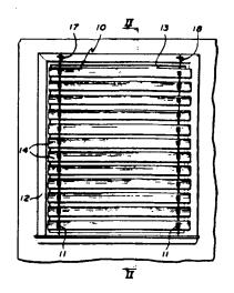
Converter for use in a location adjacent to the inside of a window to receive solar energy and change it to useful heat.
