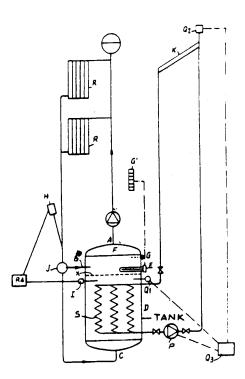
Heater comprises a container divided into upper and lower chambers by a perforated plate. The container is connected to receive heated liquid from a solar collector and deliver it to radiators or the like. The container is equipped with an electrical heating coil for further heating the liquid when the solar heat supply is inadequate.
