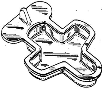
Example of a design for a food server that shows an irregular periphery in top plan and simulative ornamentation.
