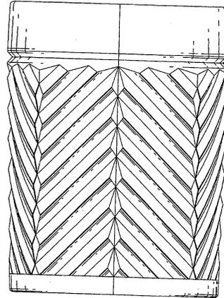
Example of a design for a glass with incised V-shaped or cutglass type pattern.
