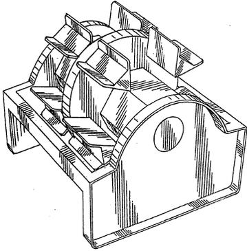
Example of a design for a condiment holder that rotates on a horizontal axis.
