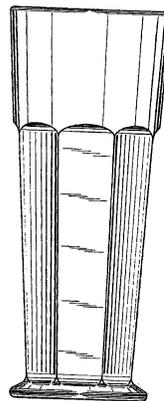
Example of a design for a glass with straight vertical ribs.
